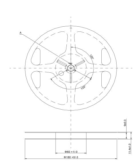
Material:Polystyrene (Conductivity) unit:mm
