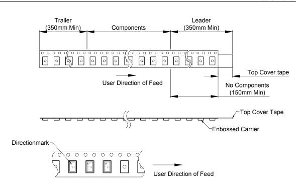
When a tape end is taken out to the front, sprocket holes becomes right hand side.
