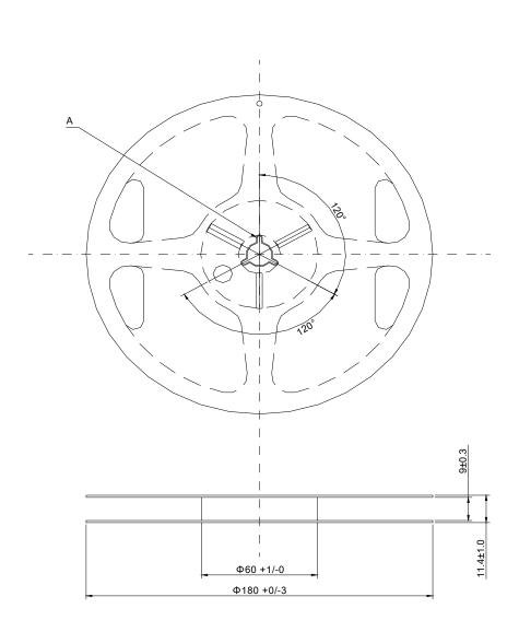
Material:Polystyrene (Conductivity) unit:mm
